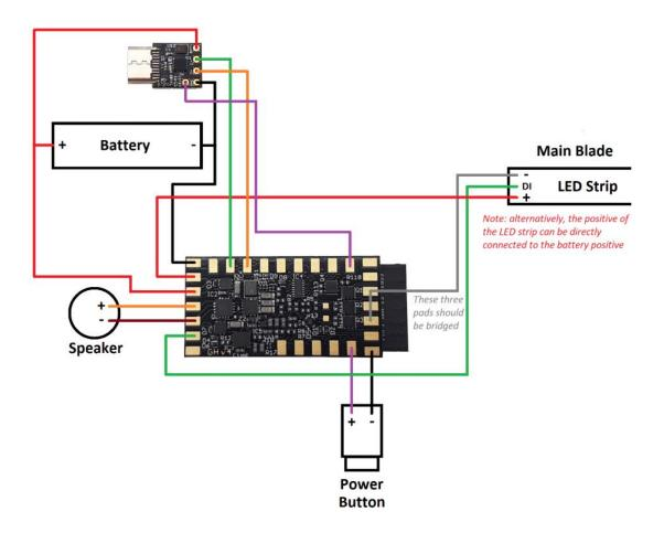
The provided wiring diagram details the connections for the Golden Harvest v4. For basic charging functionality, only the black (ground) and red (positive) wires are essential.
